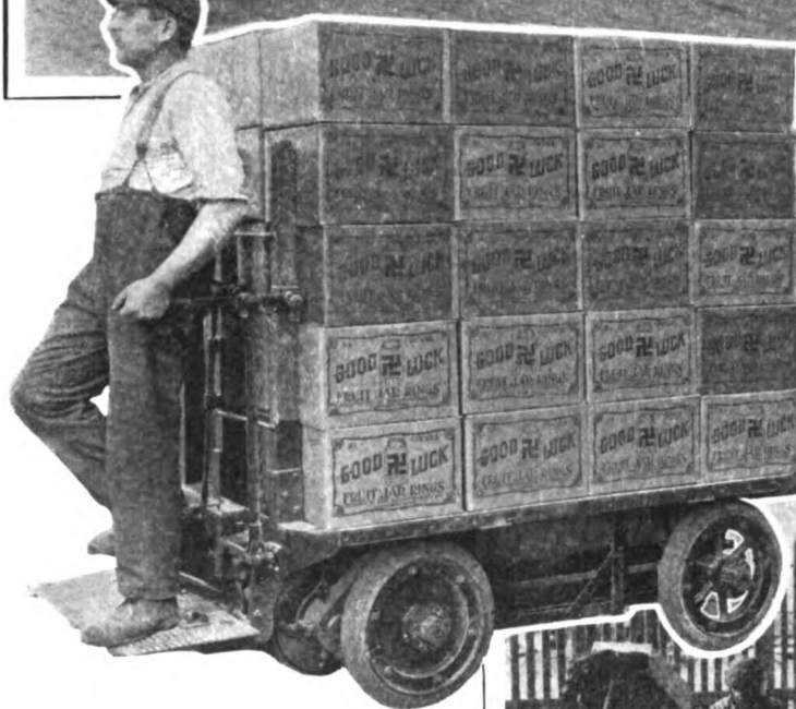
Top—Fleet of 1-ton electric freight trucks. It is these machines that allow the rapid handling of freight, thus relieving congestion and providing greater freight capacity
